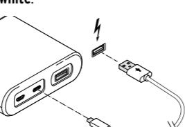
1. Connect the powerbank as shown with the enclosed USB-C/USB-A charging cable or with a micro USB/USB-A charging cable to one of the two powerbank input sockets and a USB mains adapter (not included).
