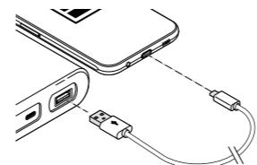
1. Connect your mobile device to the powerbank with a USB charging cable as illustrated.
